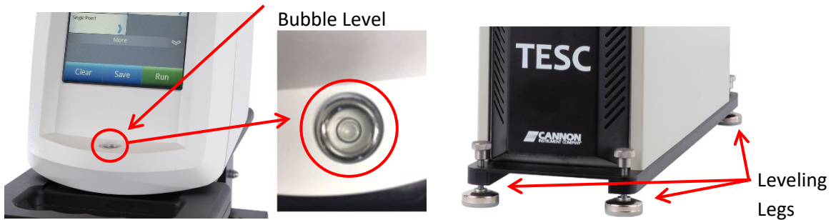
Figure 8: Bubble Level and Levelling Legs on TESC-2983
