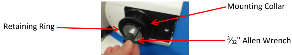
Figure 3: Removing Retaining Ring from Mounting Collar
