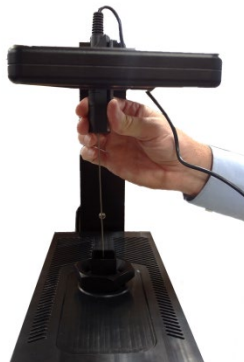
Figure 63: Temperature Probe inserted into Holder and Test Tube
