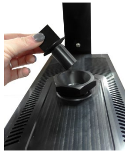
Figure 62: Inserting Temperature Probe Holder into Collar
