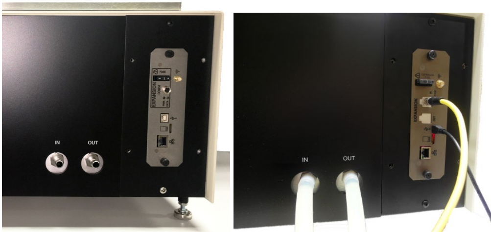
Figure 10: TE-BBR Serial Connections Back Panel and to PC (shown without and with cables)
