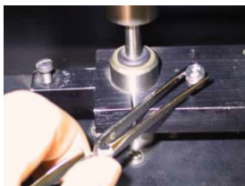
Figure 15: Placing Weight with Forceps
