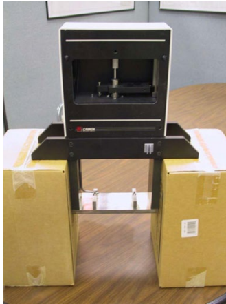
Figure 32: Supported Load Frame
