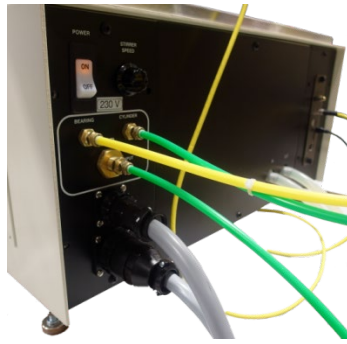
Figure 11: Dry Air/Nitrogen Connections – Control Unit
