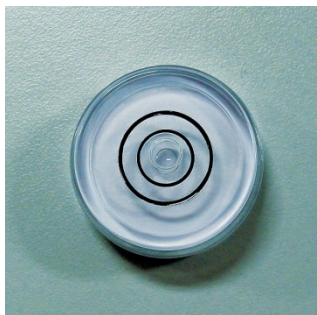
Figure 7: Bubble Level for Load Frame
