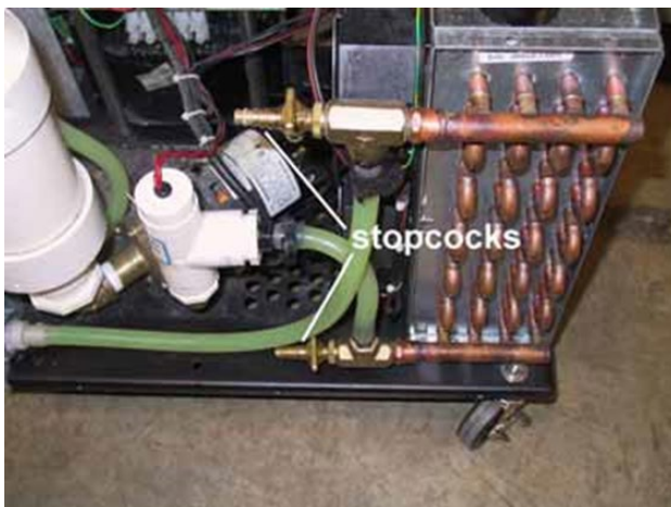
Figure 23: Exchanger with Housing Removed
