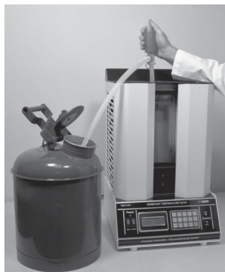
Figure 9: Siphoning bath liquid
