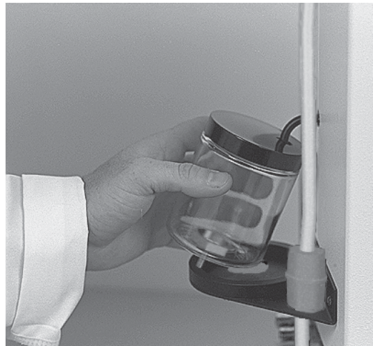
Figure 4: Overflow jar with platform and pump installed
