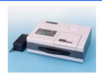
**RX-360SH** determines **total sulfur in petroleum products**, such as gas oil, fuel oil, crude oil and naphtha, using energy dispersive X-ray fluorescence (EDXRF) method, which is an accurate, non-destructive, economical and yet quick method prescribed in ISO 8754 and ASTM D4294-03.
