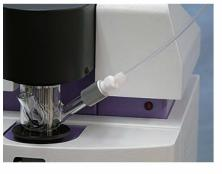
PTFE tubing connected to measuring cell for direct delivery from bottle-top dispenser for a safer aniline handling. PTFE tubing and fitting are **an option and** not provided with aap-6.
