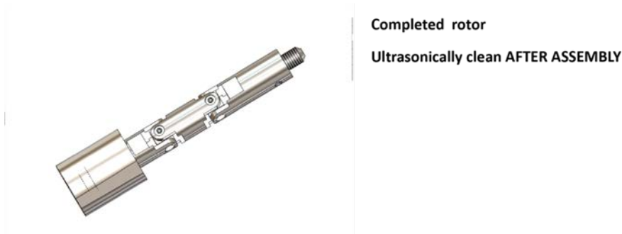
Figure 10: Clean Rotor and Stator Assembly
