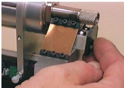
Figure 60: Insert Block under Motor Sleeve
