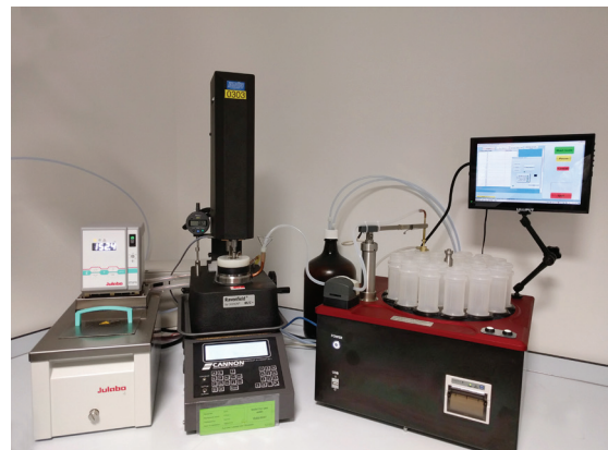
Ravenfield® BS/C+ HTHS Viscometer shown with Model DR Autosampler and temperature controlled bath
