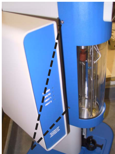
miniAV with front cover screws highlighted
