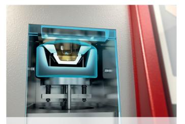
Ignition inside the continuously closed chamber formed by the sample cup and the oven plate
