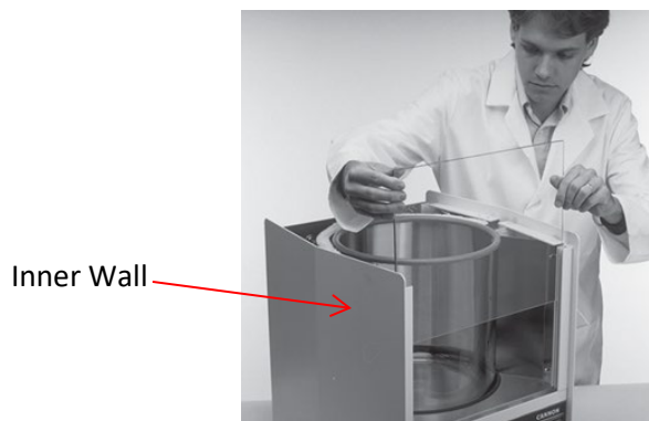
Figure 11: Placing Inner Glass Plate
