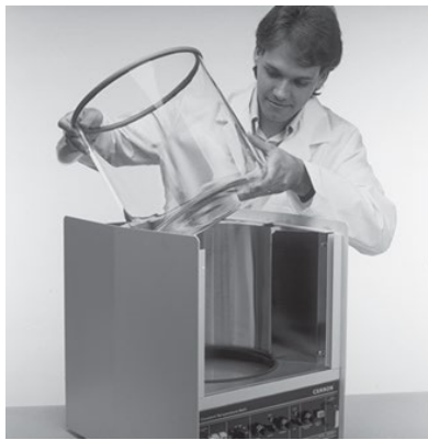
Figure 10: Installing Bath Jar
