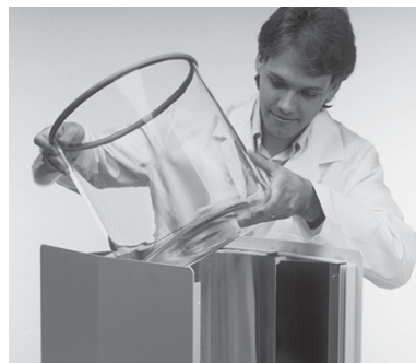
Figure 8: Installing bath jar
