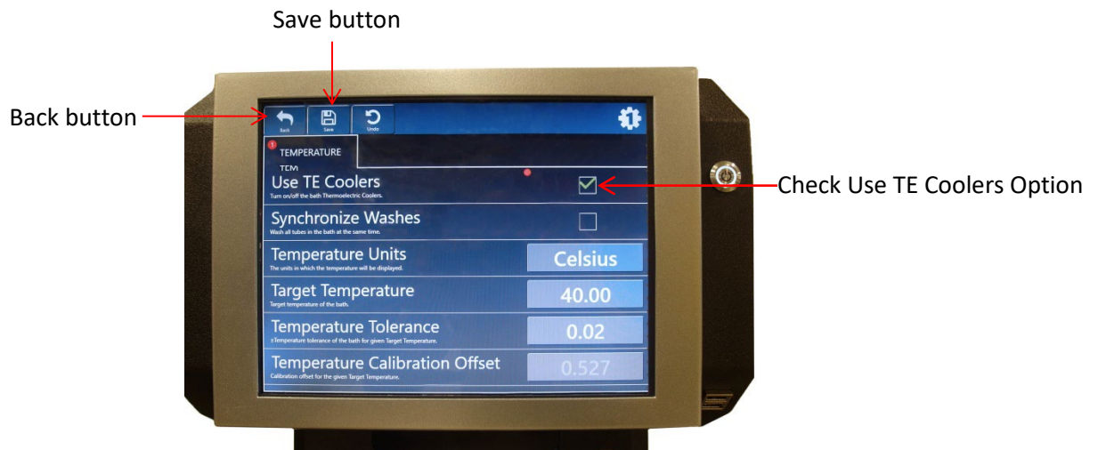
Figure 47 — Check Use TE Coolers
