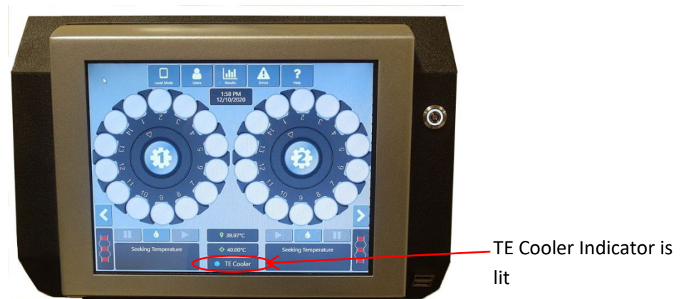
Figure 48 — TE Cooler Indicator Lit
