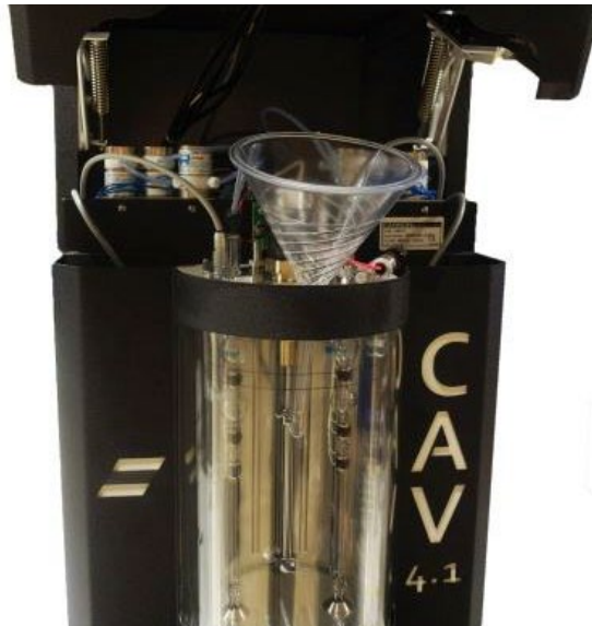
Figure 8 — Funnel Inserted into Bath Opening
