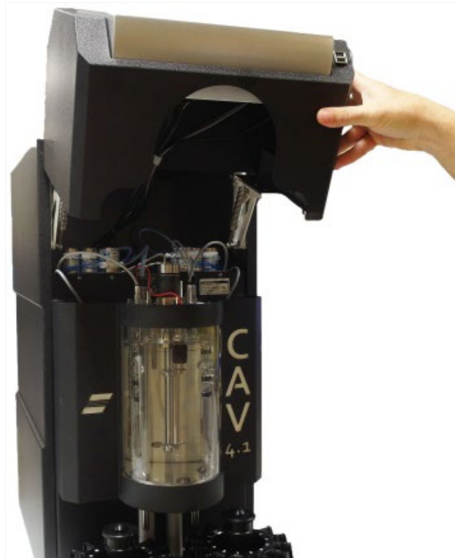
Figure 11 — Lift the CAV 4.1 Hood
