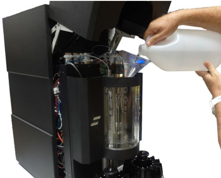
Figure 9 — Filling Bath with 10 cSt Silicone Fluid
